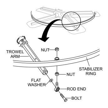
Figure 37. Trowel Arm Removal (Stabilizer Ring)
